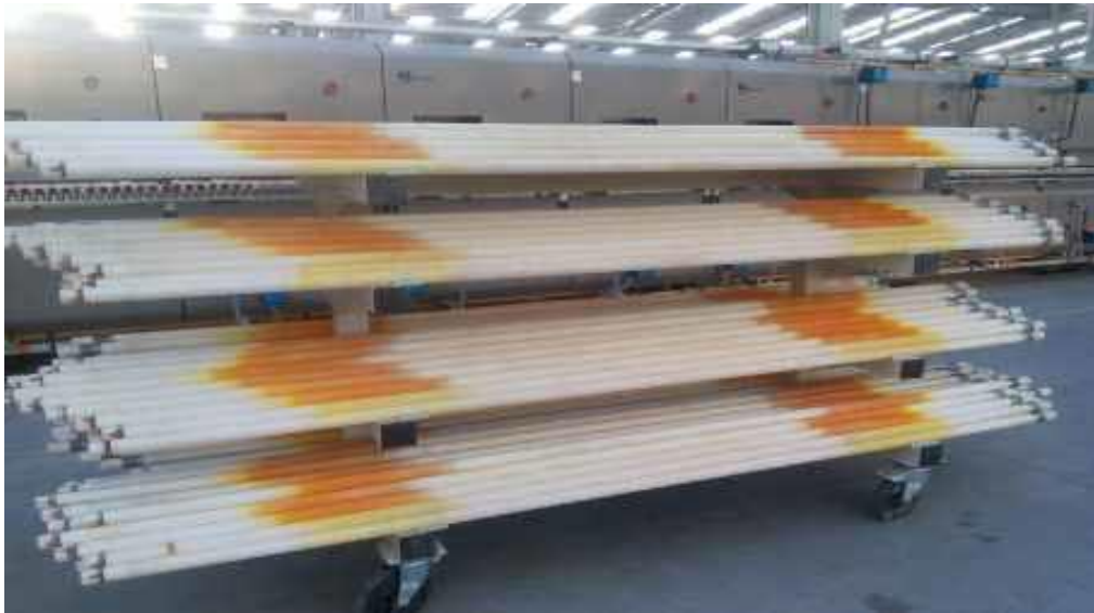
Chemically attacked rollers
