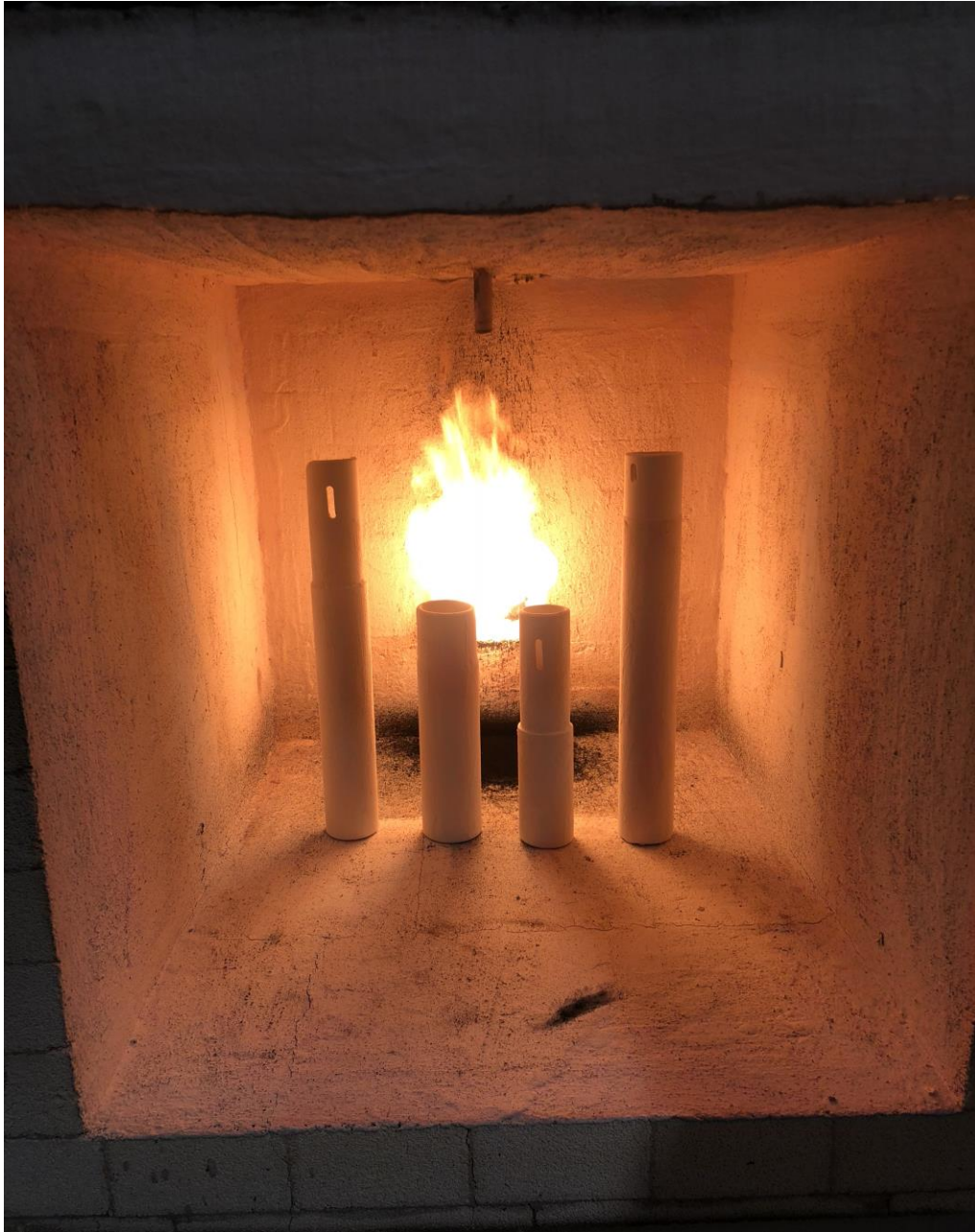
Direct heat application by raising the kiln to 1000°C in 30 minutes
